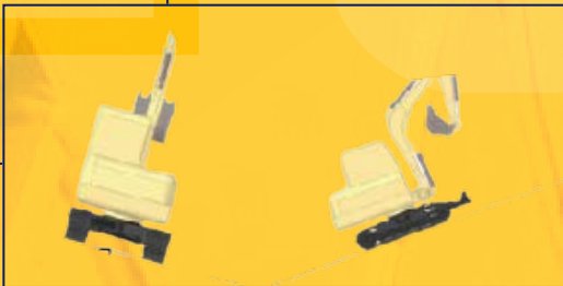
working condition of tilting & working condition of climbing
